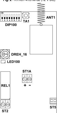
Power supply: ST1 Connection 230 V AC ST1A Connection 12 V DC
