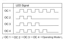
Press the transmitter button. If the Open-Collector-Receiver has memorized the code, the LED lights up for approx.
